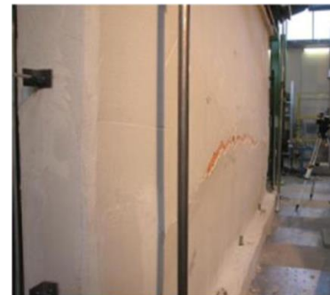
Walls Reinforced with Sisma Calce
