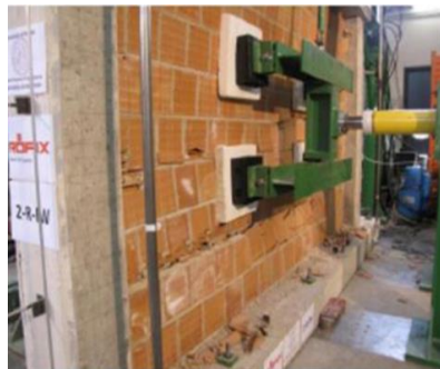
Walls Reinforced with Sisma Calce
