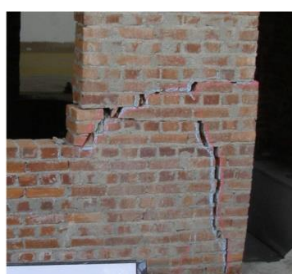
Damages on non-retrofitted model (0,35 g)
