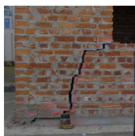
Damages on non-retrofitted model (0,35 g)
