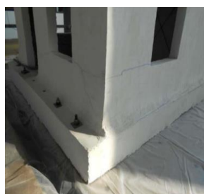
Damages on Sisma Calce retrofitted model (1,22 g)
