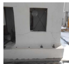
Damages on Sisma Calce retrofitted model (1,22 g)
